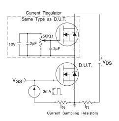
Fig 13b. Gate Charge Test Circuit
