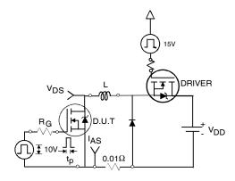
Fig 12a. Unclamped Inductive Test Circuit
