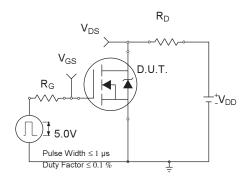
Fig 10a. Switching Time Test Circuit
