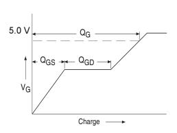
Fig 13a. Basic Gate Charge Waveform
