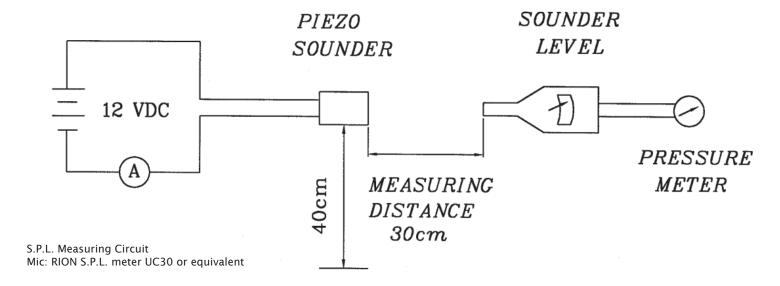
2) The current consumption and the sound pressure level are measured by using the recommended driving circuit as shown below.
