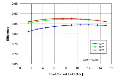
**Fig. 12:** Efficiency vs. load current lout1 and input voltage for converter mounted vertically with air flowing from pin 3 to pin 1 at a rate of 300 LFM (1.5 m/s), for lout2 = 7.5 A and Ta =  $25^{\circ}$ C.
