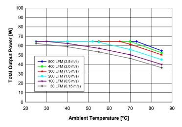
**Fig. 9:** Available output power for balanced load current (lout1 = lout2) vs. ambient air temperature and airflow rates for converter with D height pins mounted horizontally with Vin = 48 V, air flowing from pin 3 to pin 1 and maximum FET temperature  $\leq$  120°C.
