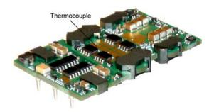
Fig. 34: Location of the thermocouple for thermal testing.
