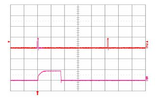
**Fig. 28:** Load current lout1 into a 10 m $\Omega$  short circuit on Vout1 during restart, with Vout2 open (no load), at Vin = 48 V. Ch2 = lout1 (20 A/div, 20 ms/div). ChB = lout1 (20 A/div, 1 ms/div) is an expansion of the on-time portion of lout1.
