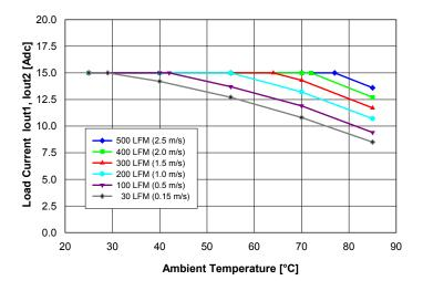
**Fig. 10:** Available balanced load current (lout1 = lout2) vs. ambient air temperature and airflow rates for converter with D height pins mounted vertically with Vin = 48 V, air flowing from pin 3 to pin 1 and maximum FET temperature  $\leq$  120°C.
