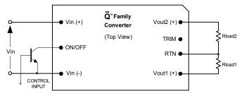
Fig. 2: Circuit configuration for ON/OFF function.
