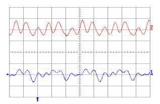
Fig. 30: Output voltage ripple at full rated load current into a resistive load on both outputs with Co = 1uF (ceramic) and Vin = 48 V. Ch2 = Vout2, Ch1 = Vout1 (both 20 mV/div). Time scale:  $1 \mu$ s/div.
