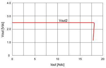
**Fig. 27:** Output voltage Vout2 vs. load current lout2 showing current limit point and converter shutdown point. When Vout2 is in current limit, Vout1 is not affected until Vout2 reaches the shut-down threshold equal to Vout1 - 0.6 V. Input voltage has almost no effect on Vout2 current limit characteristic.
