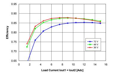
**Fig. 16:** Efficiency vs. balanced load current (lout1 = lout2) and input voltage for converter mounted vertically with air flowing from pin 3 to pin 1 at a rate of 300 LFM (1.5 m/s) and Ta =  $25^{\circ}$ C.
