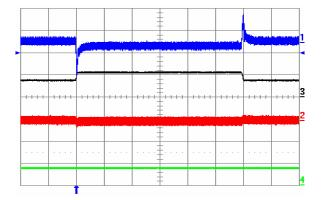
**Fig. 20:** Output voltage response to lout1 load current stepchange of 3.75 A (50%-75%-50%) at lout2 = 7.5 A and Vin = 48 V. Ch1 = Vout1 (50 mV/div), Ch2 = Vout2 (50 mV/div), Ch3 = lout1 (10 A/div.), Ch4 = lout2 (10 A/div.). Current slew rate: 0.1 A/µs, Co = 10 µF tantalum + 1 µF ceramic. Time scale: 0.5 ms/div.
