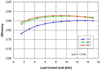
**Fig. 14:** Efficiency vs. load current lout2 and input voltage for converter mounted vertically with air flowing from pin 3 to pin 1 at a rate of 300 LFM (1.5 m/s), for lout1 = 7.5 A and Ta =  $25^{\circ}$ C.
