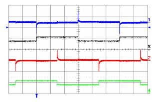
**Fig. 25:** Output voltage response to both lout1 and lout2 (out of phase) load current step-change of 3.75 A (50%-75%-50%) at Vin = 48 V. Ch1 = Vout1 (100 mV/div), Ch2 = Vout2 (100 mV/div), Ch3 = lout1 (10 A/div.), Ch4 = lout2 (10 A/div.). Current slew rate: 5 A/ $\mu$ s, Co = 300  $\mu$ F tantalum + 1  $\mu$ F ceramic. Time scale: 1 ms/div.
