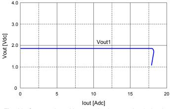
**Fig. 26:** Output voltage Vout1 vs. load current lout1 showing current limit point and converter shutdown point. When Vout1 is in current limit, Vout2 is not affected until Vout1 reaches the shut-down threshold of 60% of its nominal value. Input voltage has almost no effect on Vout1 current limit characteristic.
