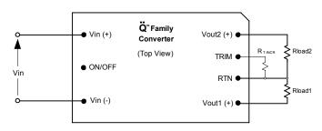
Fig. 3: Configuration for increasing output voltage.
