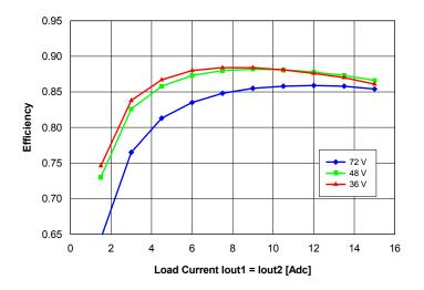
**Fig. 17:** Efficiency vs. balanced load current (lout1 = lout2) and input voltage for converter mounted horizontally with air flowing from pin 3 to pin 1 at a rate of 300 LFM (1.5 m/s) and Ta =  $25^{\circ}$ C.
