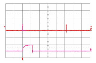
**Fig. 29:** Load current lout2 into a 10 m $\Omega$  short circuit on Vout2 during restart, with Vout1 open (no load), at Vin = 48 V. Ch2 = lout2 (20 A/div, 20 ms/div). ChB = lout2 (20 A/div, 1 ms/div) is an expansion of the on-time portion of lout2.
