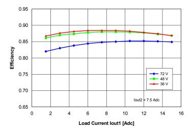
**Fig. 13:** Efficiency vs. load current lout1 and input voltage for converter mounted horizontally with air flowing from pin 3 to pin 1 at a rate of 300 LFM (1.5 m/s), for lout2 = 7.5 A and Ta =  $25^{\circ}$ C.
