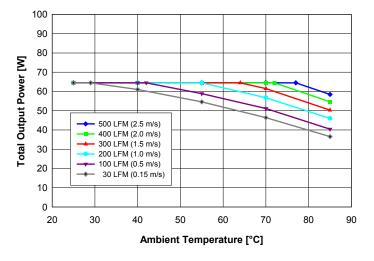
**Fig. 8:** Available output power for balanced load current (lout1 = lout2) vs. ambient air temperature and airflow rates for converter with D height pins mounted vertically with Vin = 48 V, air flowing from pin 3 to pin 1 and maximum FET temperature  $\leq$  120°C.
