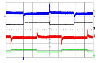
**Fig. 24:** Output voltage response to both lout1 and lout2 (out of phase) load current step-change of 3.75 A (50%-75%-50%) at Vin = 48 V. Ch1 = Vout1 (50 mV/div), Ch2 = Vout2 (50 mV/div), Ch3 = lout1 (10 A/div.), Ch4 = lout2 (10 A/div.). Current slew rate: 0.1 A/µs, Co = 10 µF tantalum + 1 µF ceramic. Time scale: 1 ms/div.
