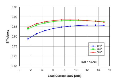
**Fig. 15:** Efficiency vs. load current lout2 and input voltage for converter mounted horizontally with air flowing from pin 3 to pin 1 at a rate of 300 LFM (1.5 m/s), for lout1 = 7.5 A and Ta =  $25^{\circ}$ C.
