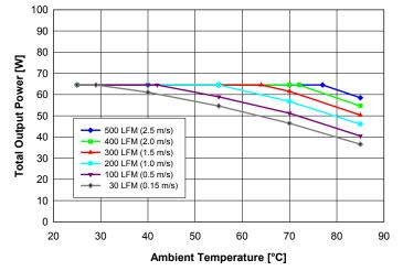
**Fig. 1:** Available output power vs. ambient air temperature and airflow rates for QD48T018025 converter with D height pins mounted vertically with air flowing from pin 3 to pin 1, MOSFET temperature  $\leq 120^{\circ}$ C, Vin = 48 V and balanced load on both outputs (lout1 = lout2).
