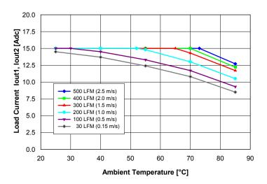
**Fig. 11:** Available balanced load current (lout1 = lout2) vs. ambient temperature and airflow rates for converter with D height pins mounted horizontally with Vin = 48 V, air flowing from pin 3 to pin 1 and maximum FET temperature  $\leq$  120°C.
