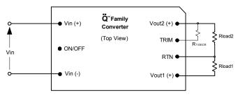
Fig. 4: Configuration for decreasing output voltage.
