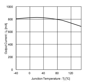
Figure 12. Output Current vs Temperature
