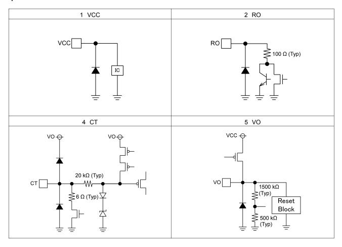
Figure 23. I / O equivalence circuits
