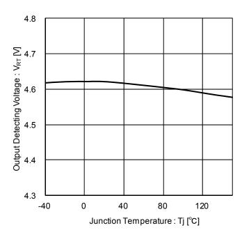
Figure 17. Output Detecting Voltage vs Temperature (RO: 10  $k\Omega$  pull-up to VO)
