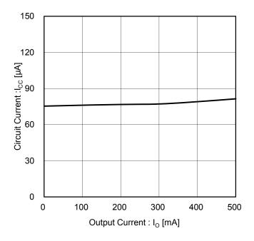
Figure 9. Circuit Current vs Output Current
