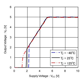
Figure 6. Output Voltage vs Supply Voltage (at Low supply voltage,  $R_L = 25 \Omega$ )
