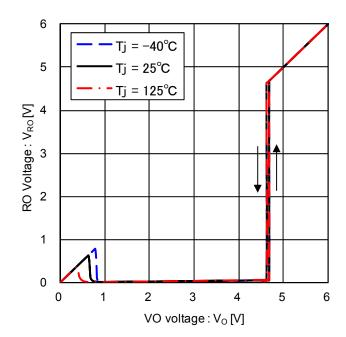
Figure 16. RO Voltage vs VO Voltage (RO: 10 k $\Omega$  pull-up to VO)
