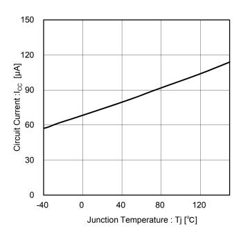
Figure 10. Circuit Current vs Temperature
