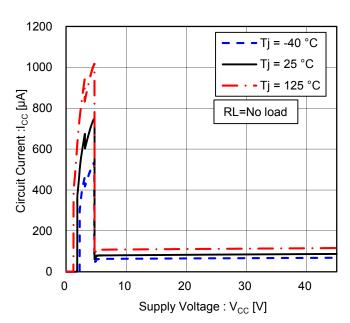
Figure 8. Circuit Current vs Supply voltage
