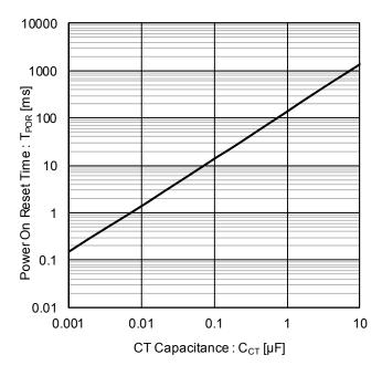
Figure 19. Power on Reset Time vs CT Capacitance
