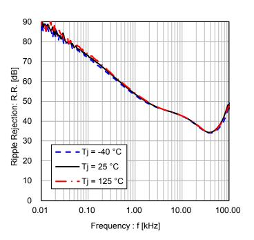
Figure 14. Ripple Rejection (ein=1Vrms, I<sub>OUT</sub>=100mA)
