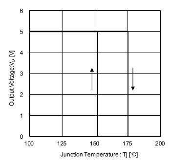
Figure 15. Output Voltage vs Temperature (Thermal Shut Down)
