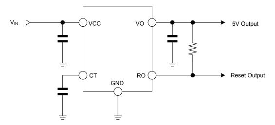
Figure 2. Application Circuit
