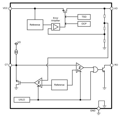
Figure 4. Block Diagram
