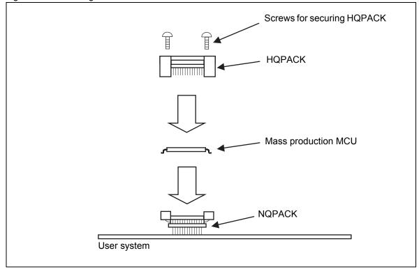
Figure 6-1. Mounting a Mass Production MCU
