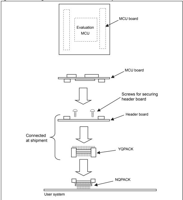
Figure 5-2. Connecting MCU Board/Header Board to User System
