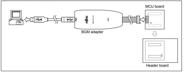
Figure 1-1. System Configuration
