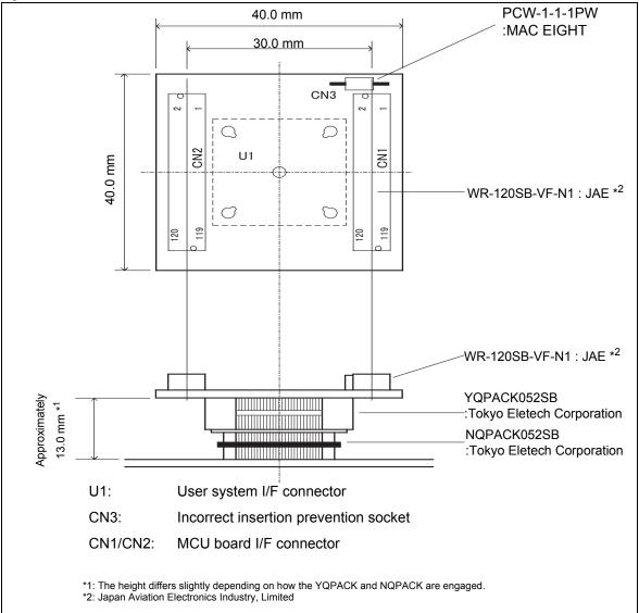
Figure 4-1. Header Board Dimensions
