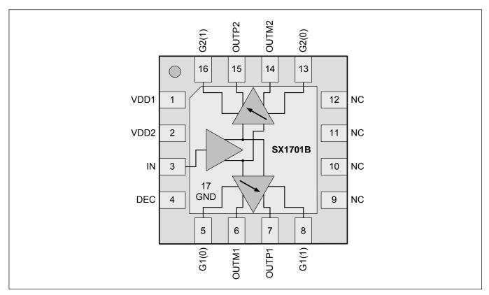
Figure 1. Simplified block diagram of the SX1701B.
