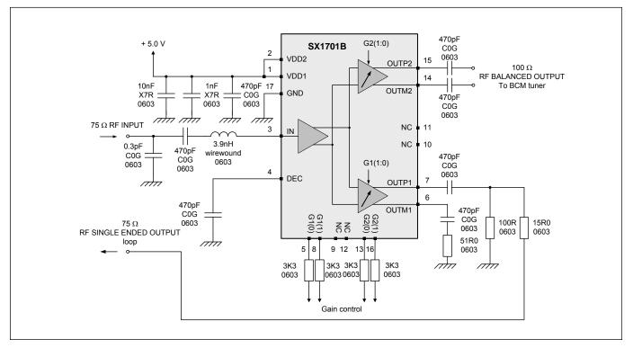
Figure 5. Differential output with loop-through.
