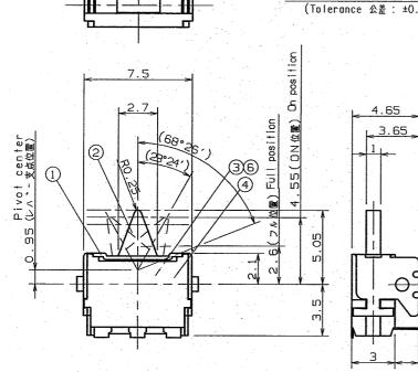
□ Release point :inclination 15 max. \*After operating several times, measure of lever position. Operating speed : 200 mm/s □ レリース、位置のレハ、一傾き --- 15 以下
