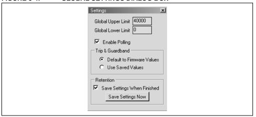
The global limit area allows the minimum and maximum values for all of the bar graphs to be globally set manually. The values must be in the range from 0 to 65535. Enter a value in the text box and press <Enter> for the value to take effect. Notice that changing this setting overrides any auto-scaling that has been performed.
