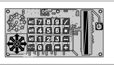
Nine of the A/D channels are used to monitor the numeric keypad switches (S1 through S12 and S21 through S27), arranged in a 4x5 array. Each "switch" is composed of interleaved conductors from two channels. The location of the touched key is determined by a simultaneous capacitance change on any two channels.
